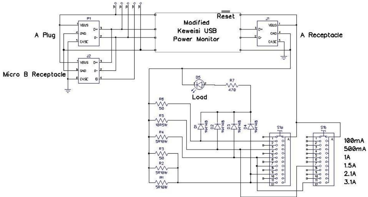
USB Power Monitor & Dummy Load
