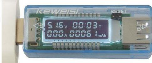
I picked the Keweisi Charger Doctor it displays: volts, milliamps, milliamp hours and elapse time. It only costs a few dollars. A nice feature is the total is stored in nonvolatile memory so the result is not lost even if power is removed. A reset button clears elapsed time and mAh.
