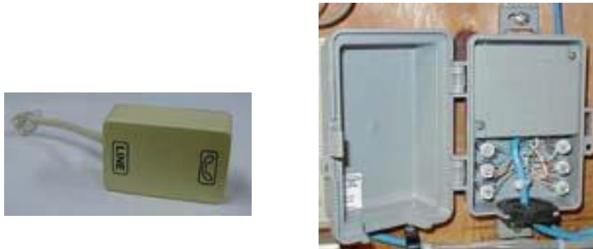
Figure 16 Inline Filter and Whole House POTS/DSL Splitter
