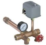
There are a lot of devices connected at the pressure tank so a special fitting called a pressure tank tee is used. Water from the pump enters from either the left or right, and exits to the house on the opposite side. The tee is plumbed into the pressure tank so when pump is on water flows into the tank and as water is drawn with the pump is off air in the tank maintains pressure.
