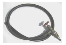
Using hose bibs rather than ball valve drain fittings makes it easy to use compressed air to blow out the system. I made up a simple adapter consisting of a washing machine hose, valve and quick connect air fitting. I used an old globe valve to adapt hose connection to pipe thread. Works great for blowing water out of the system. It also came in handy when I was building the various systems as I could pressurize them with air, rather than water for leak testing.
