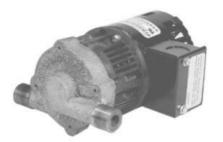
To capture more energy and minimize how often the preheat tank PTRV dumps excess hot water I installed a small <u>circulator pump</u> plumbed between electric water heater hot-water outlet and pre heat tank cold water inlet. One of the functions of the <u>wood heat</u> <u>controller</u> is to monitor preheat tank temperate to control the pump. The pump is specifically designed for high temperature applications.
